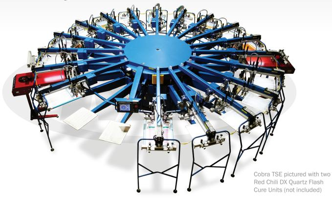
The COBRA TSE™ series of presses provides operators with timesaving features needed for quick setups—electric printheads with electronic controls, tool-free squeegee/floodbar angle adjustment with pneumatic clamps, pneumatic screen frame locks, and independent squeegee/flood speeds with digital displays. Cobra TSE also features a revised, robust, smooth and quiet flat indexing system.
